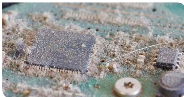
Buildup of dust on crucial internal parts can have a major impact on overall performance
