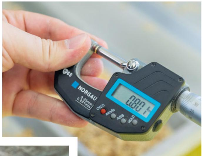
A final quality check of the thickness of an oat flake is carried out in the laboratory.
