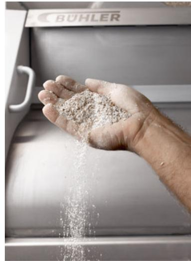
After grinding, the desired particle size is achieved. The intermediate material is now ready to be separated into the fractions.
