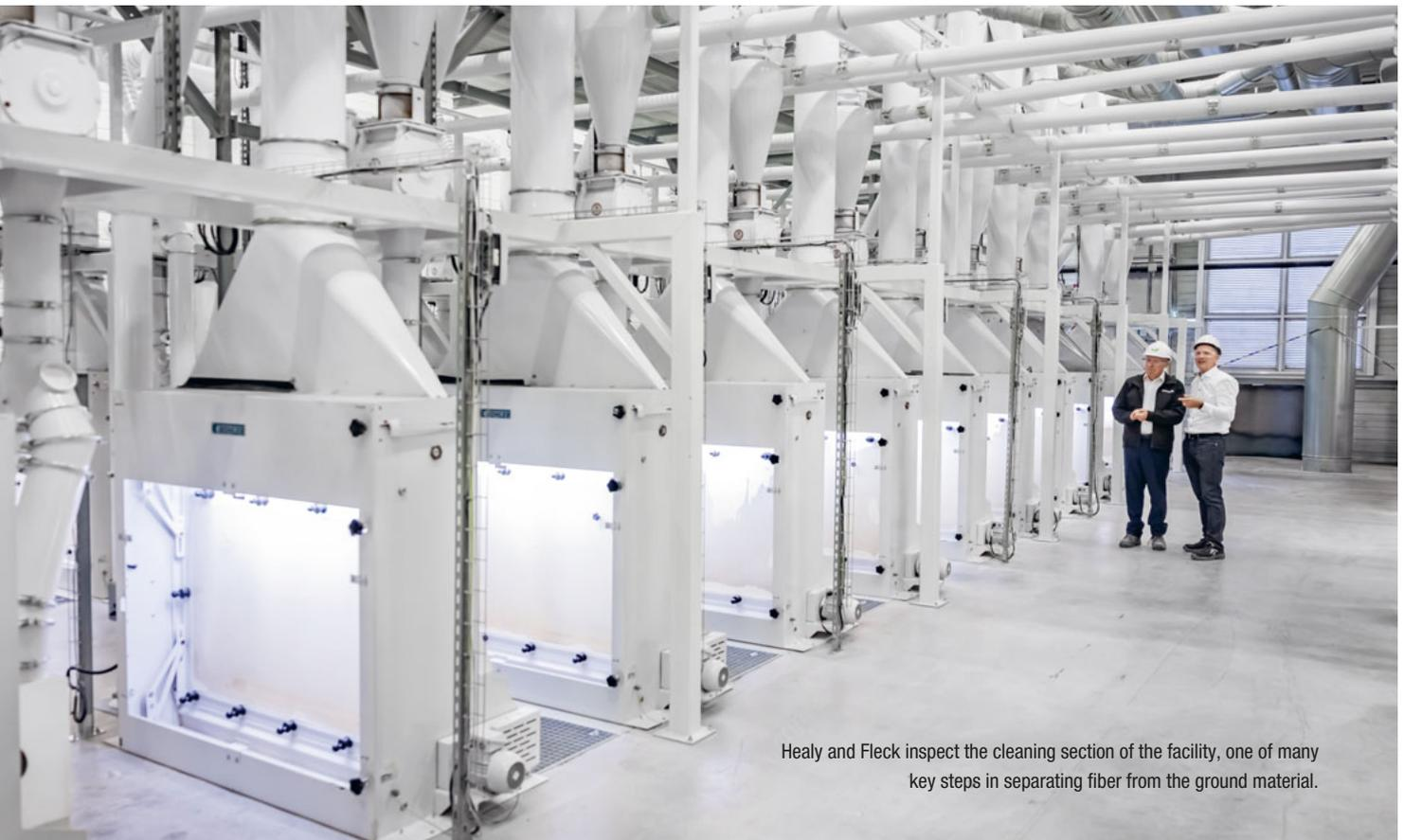
Healy and Fleck inspect the cleaning section of the facility, one of many key steps in separating fiber from the ground material.
