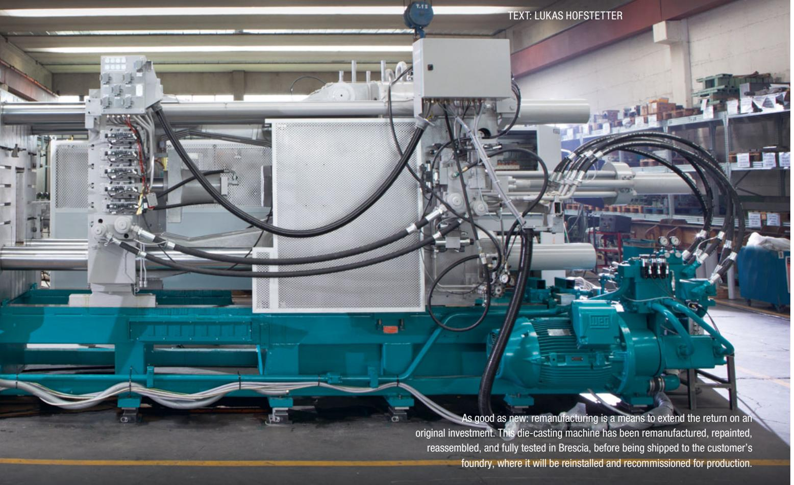
As good as new: remanufacturing is a means to extend the return on an original investment. This die-casting machine has been remanufactured, repainted, reassembled, and fully tested in Brescia, before being shipped to the customer's foundry, where it will be reinstalled and recommissioned for production.
