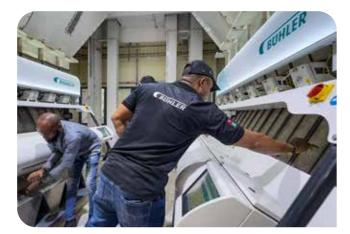
The fully automated mill is equipped with Bühler's state-of-the-art rice processing machinery, including a harvest dryer - a rarity in Nigeria which enables paddy with higher moisture contents to be dried sufficiently to be safely stored, ensuring that none of the crop is wasted. The mill has been up and running for three years now and is the largest rice production facility in sub-Saharan Africa, with an annual capacity of around 2.5 million 50 kg bags of rice.
