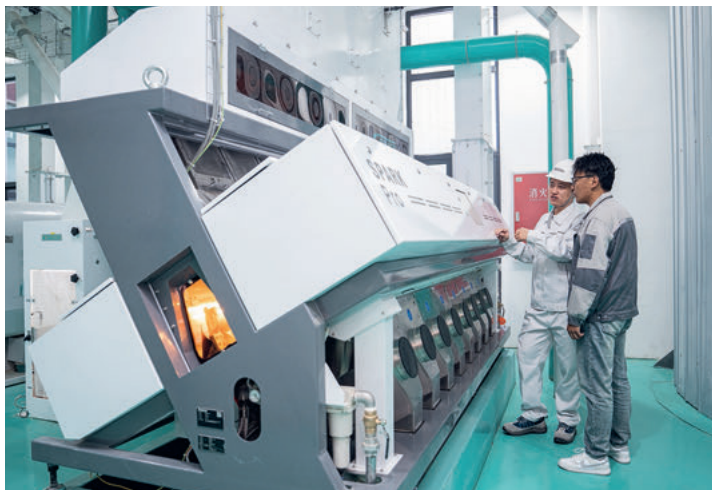
The Bühler SORTEX SPARK Pro optical sorter detects and removes defective grains, ensuring high product quality and food safety.
