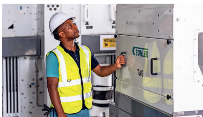
A glimpse into the heart of the RimoMalt: the process chamber where germination and kilning are combined.
