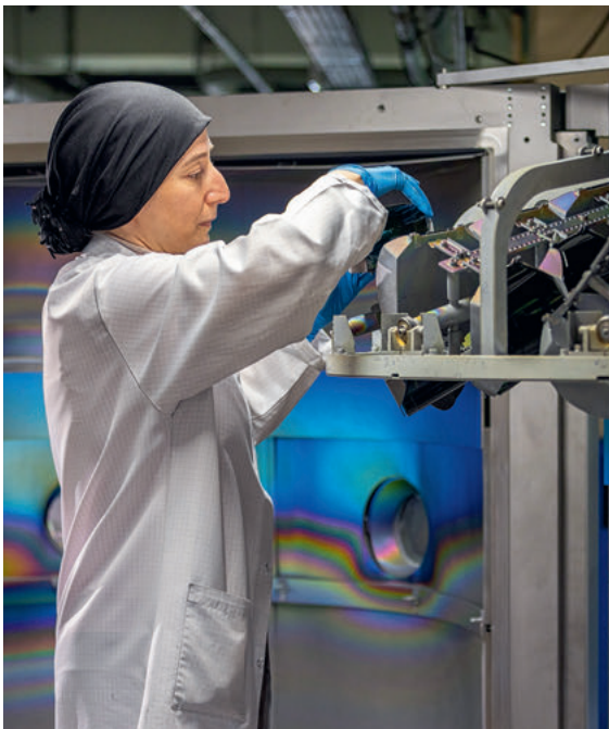
The curved polycarbonate sport lenses are inspected after the physical vapor deposition process.
