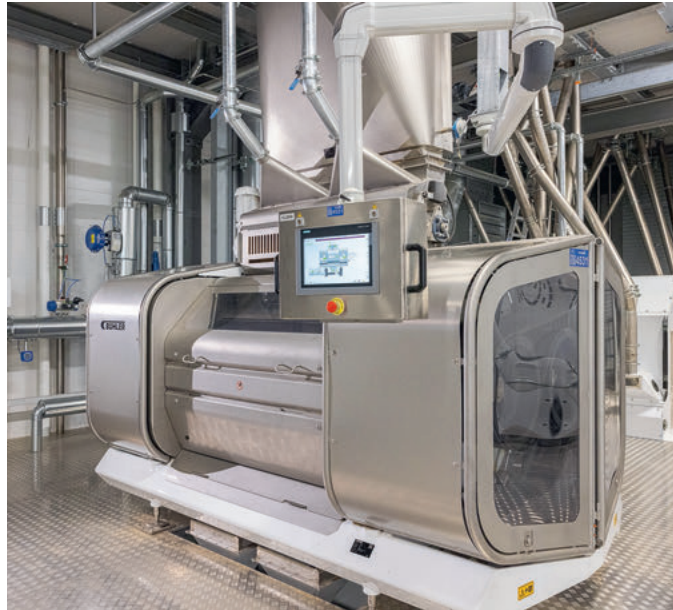
The PolyFlake flaking mill is designed to meet the highest food safety standards while ensuring consistent product quality.
