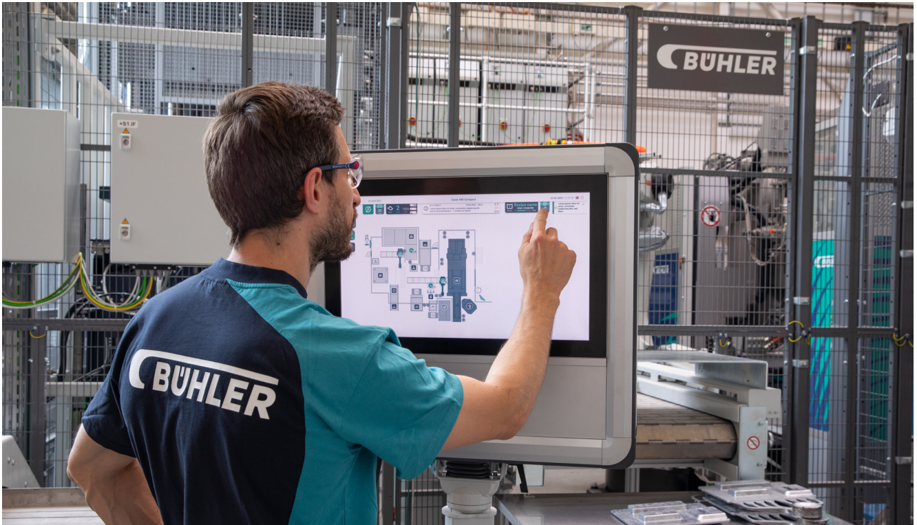
SmartCMS allows you to control the entire die-casting cell from a centralized location.
