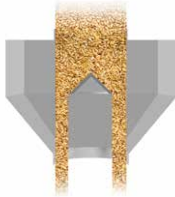
Other principles Measuring only parts of mass stream and estimating mass flow
