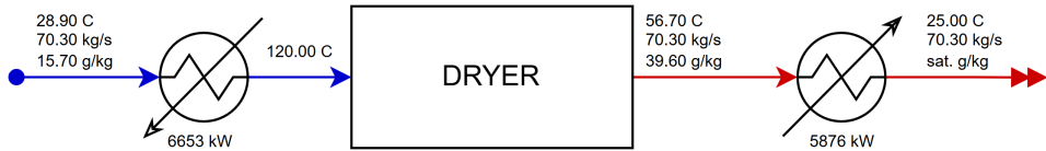
Figure 10. Representation of the chosen drying process with fresh air (blue) and exhaust air (red).
