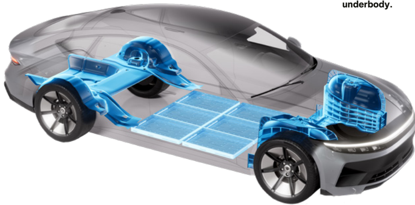
Megacasting parts in a car: rear underbody, battery tray, and front underbody.
