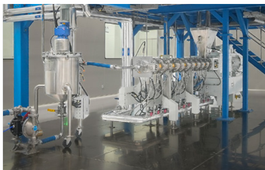
At the core of Bühler's battery mixing system is a twin-screw extruder.
