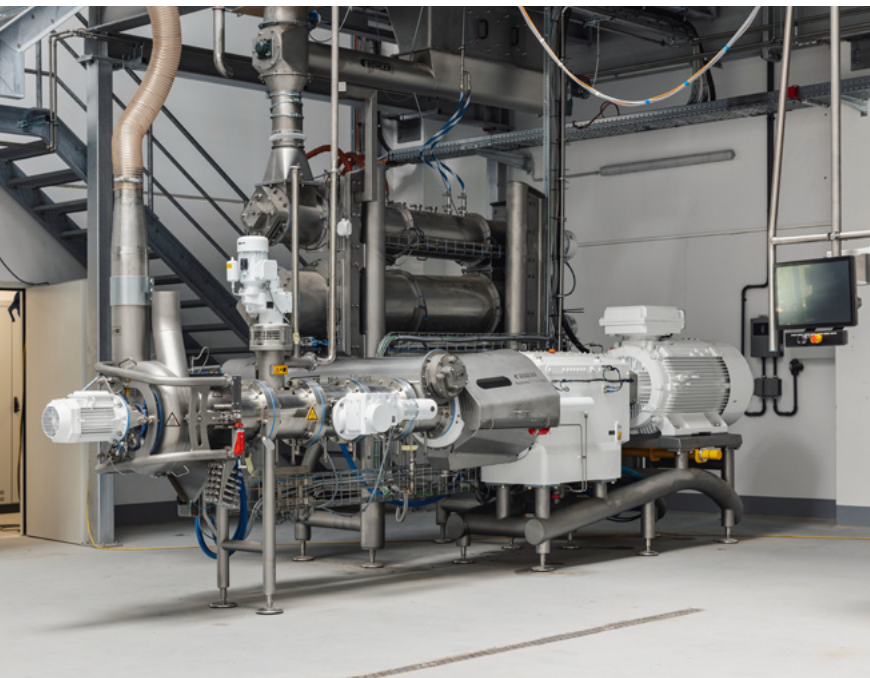
The hygienic design of the Nutrex 7 Series twin-screw extruder shortens cleaning times.
