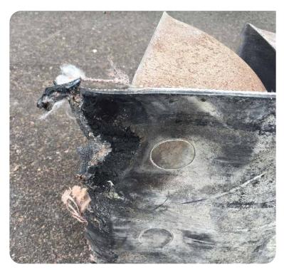
A torn belt in the elevator can have serious consequences during ongoing operation. It results in unplanned maintenance work and expenses and very high additional repair costs.
