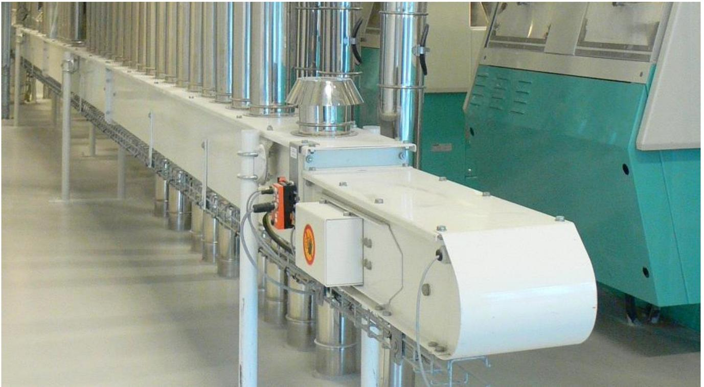
**Chain conveyor – Stainless steel conveyors as well as transportation tasks of finished products in processing plants.**
