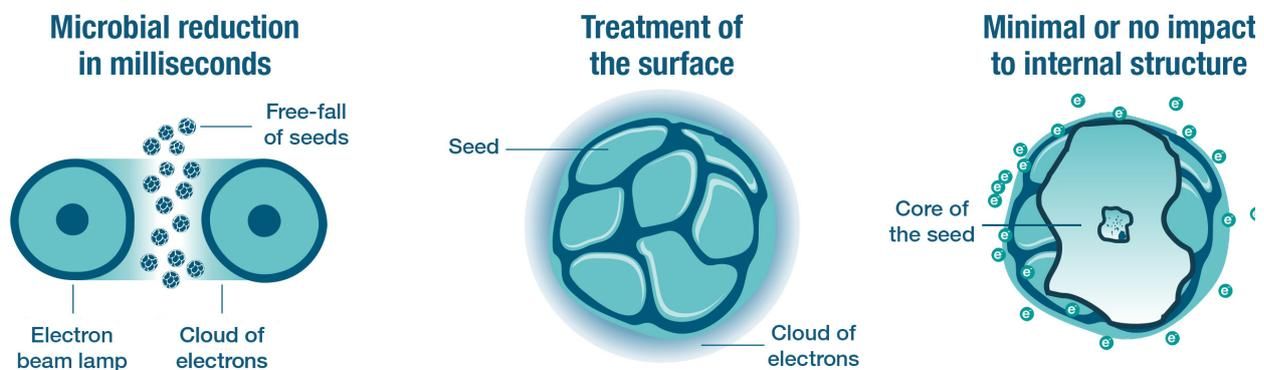
**Figure 2.** The principle of Laatu. The curtain of seeds free-fall through low energy electron beam lamps where each seed is homogeneously exposed to a cloud of electrons. Due to the low energies of the electrons, only surface of the seed is treated, preserving the internal quality of the seed.
