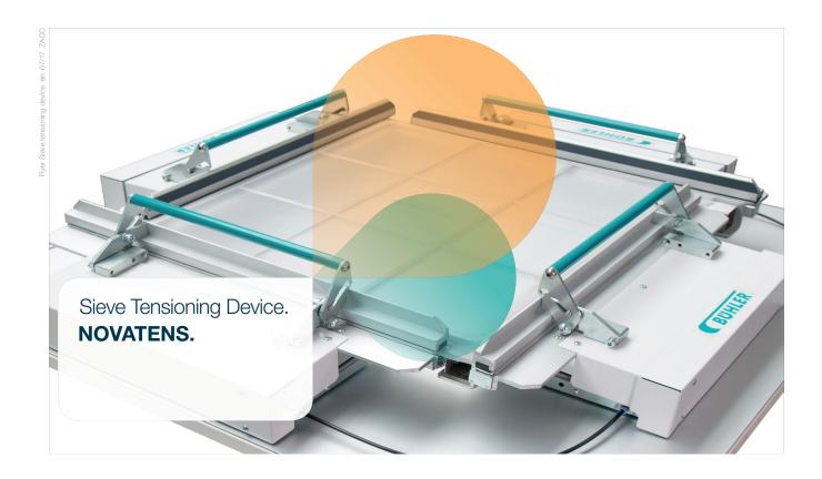
NOVATENS is a pneumatic sieve tensioning device for covering the insertion frames of plansifters and purifiers. Due to its high and even clamping force the best sieve tensioning results are achieved.
