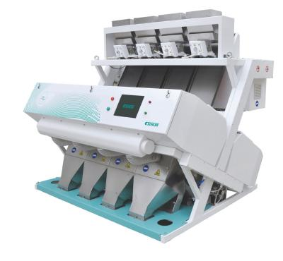
Indeed, he shares the company's notable cost savings as a result of using the optical sorter. "In general, without an optical sorter we would expect a physical loss of 0.2% of the coffee (approximately 15.000 USD), but with the optical sorter, the losses are much closer to 0.0%.
