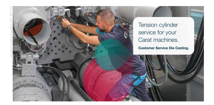
Many of the Carat die-casting machines have been in operation for years in harsh foundry conditions, producing millions of parts. An integral part of the Carat are the tension cylinders, which ensure the locking force on our two-platen solution. As they are in constant movement for every cycle, we recommend an exchange at the right time to prevent unplanned surprises.
