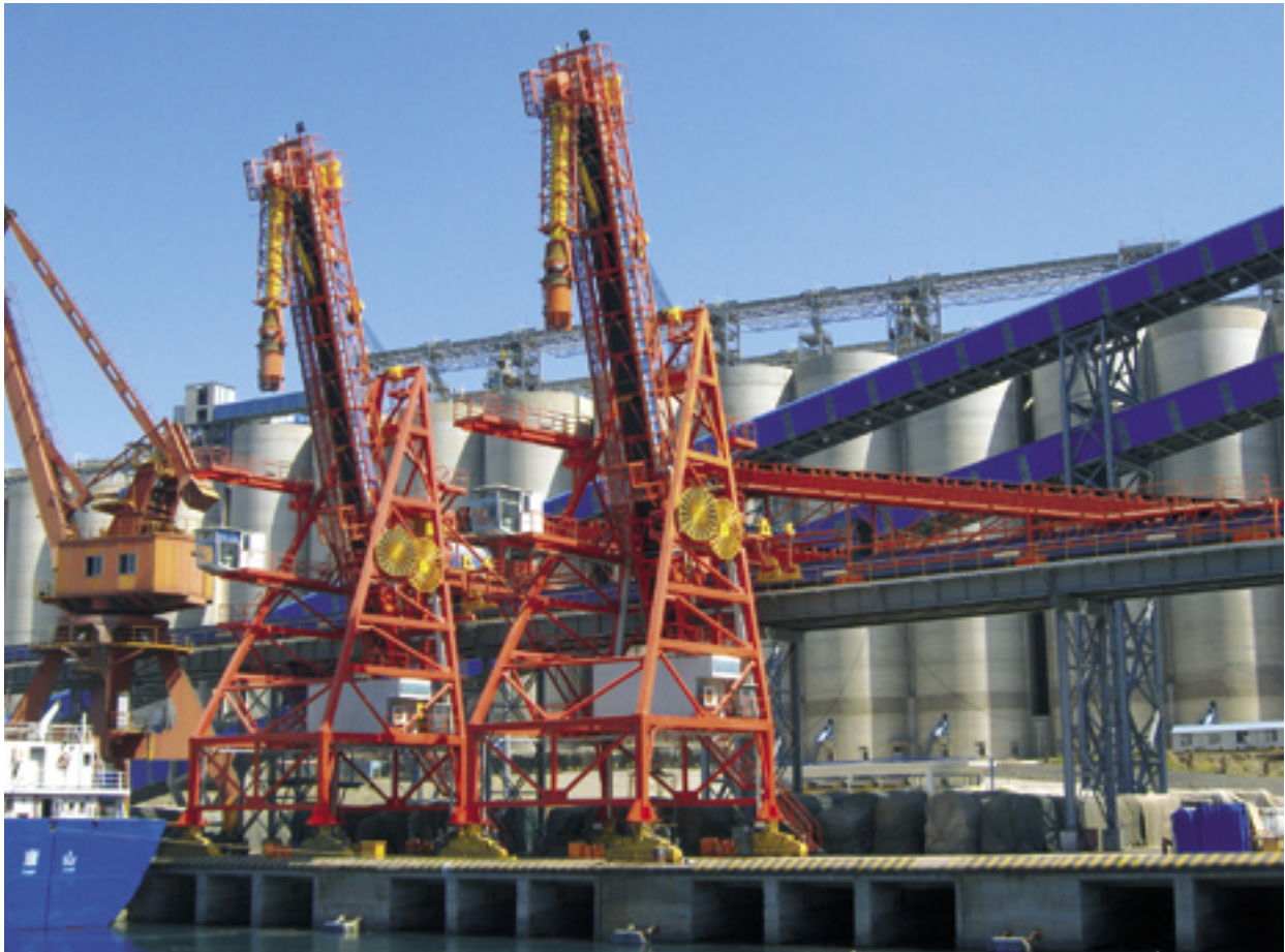
Dalian Beiliang Grain Terminal, China. Ship loaders, 2 \times 1000 t/h.
