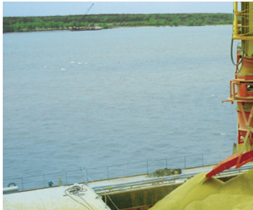
RGLZ-1000 dust suppressor, designed for loading throughputs up to 2000 t/h of grain. The dust suppressor is provided with a distribution chute that can be rotated 360° and therefore allows optimal filling of the hold.
