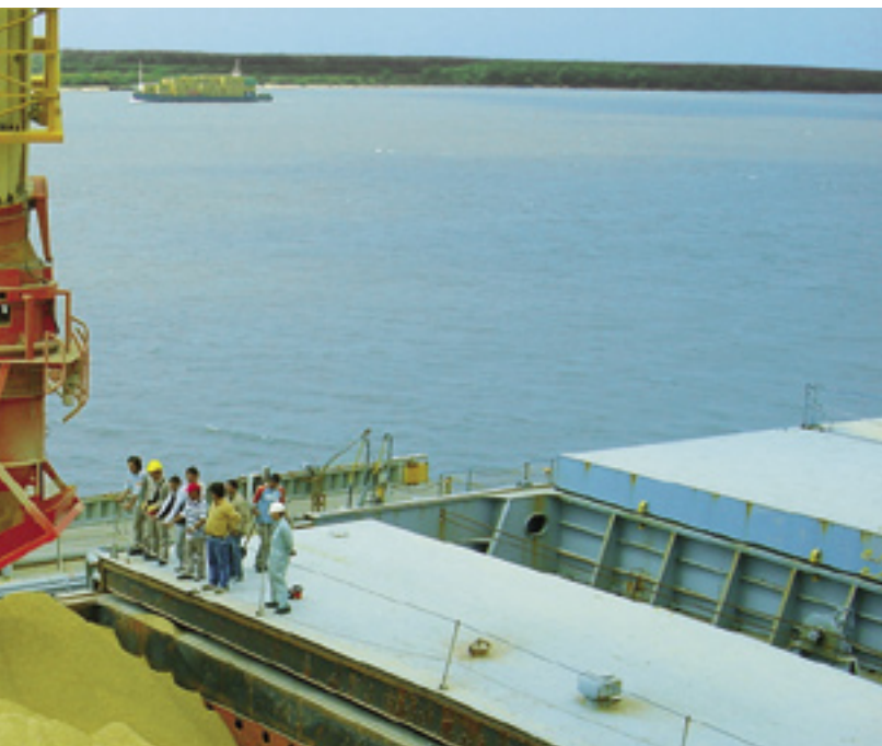
Lantmännen, Moss, Norway. Stationary ship loader 300 t/h with dust suppressor.
