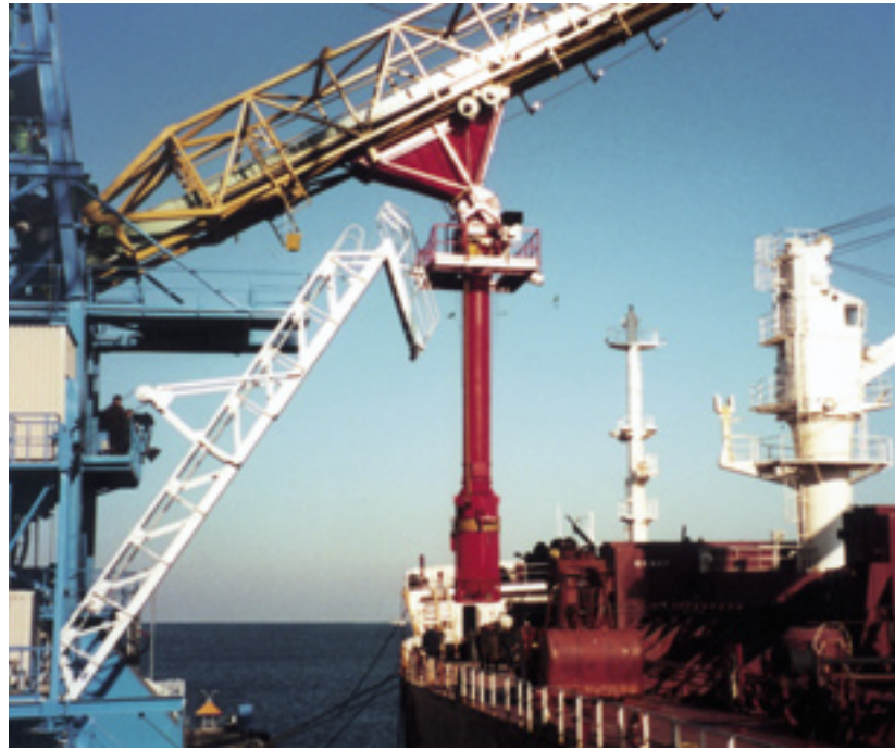
Muuga Grain Terminal, Tallinn, Estonia. Ship loader with RGLZ dust suppressor.
