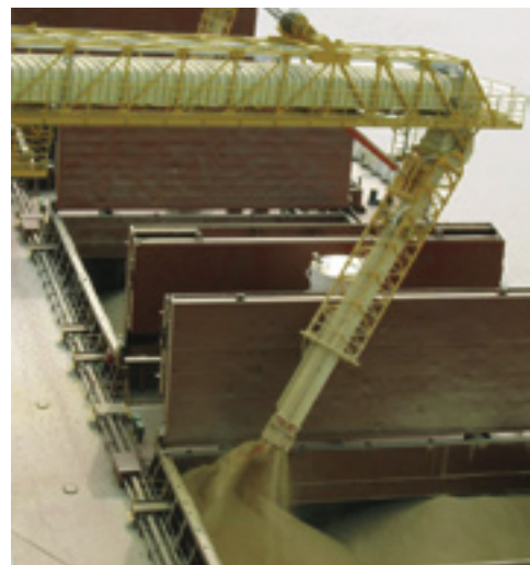
Large kick angle allows optimal filling of the holds.
