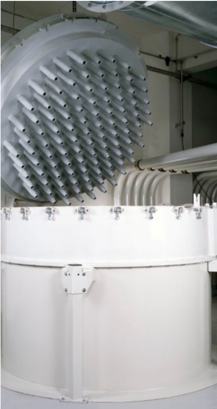
Low-Pressure Airjet-Filter MVRT. Top Removal.
