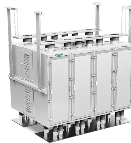
Arenit Plus plansifter: safe sifting, sorting and classification of floury products.
